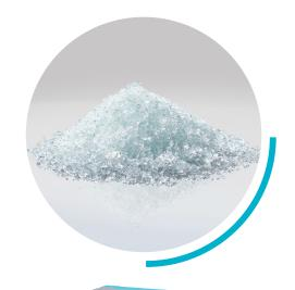
2 Crystal Clear, the media made of glass crystals, provides ultra-fine filtration.
